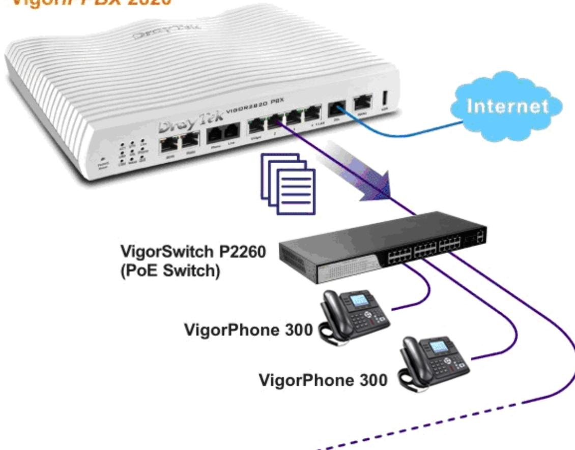
1. Configure the extension number and password for each IP phone on VigorIPPBX 2820. You can configure extensions from IP PBX Wizard.
