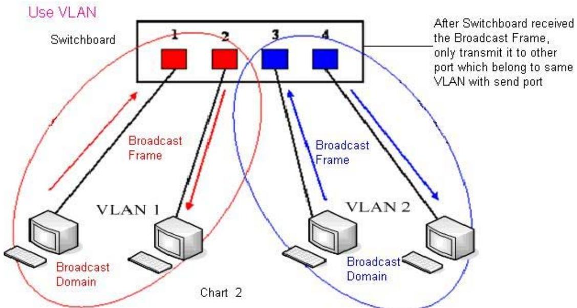
In chart 2, red and blue circles indicate two different VLANs in the switch, and port 1 and port 2 belong to red VLAN, port 3 and port 4 belong to blue VLAN. If a broadcast frame is sent out from port 1, the switch will transmit it to port 2, the other port in the red VLAN and not transmit it to port 3 and port 4 in blue VLAN. By this means, VLAN divides the broadcast domain via restricting the range of broadcast frame transmission.
