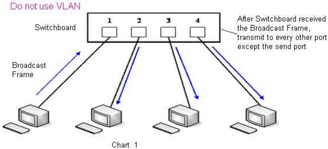
In chart 1, there is a switch without setting VLAN. Any broadcast frame will be transmitted to the other ports except the send port. For example, a broadcast information is sent out from port 1 then transmitted to port 2,3 and 4.
